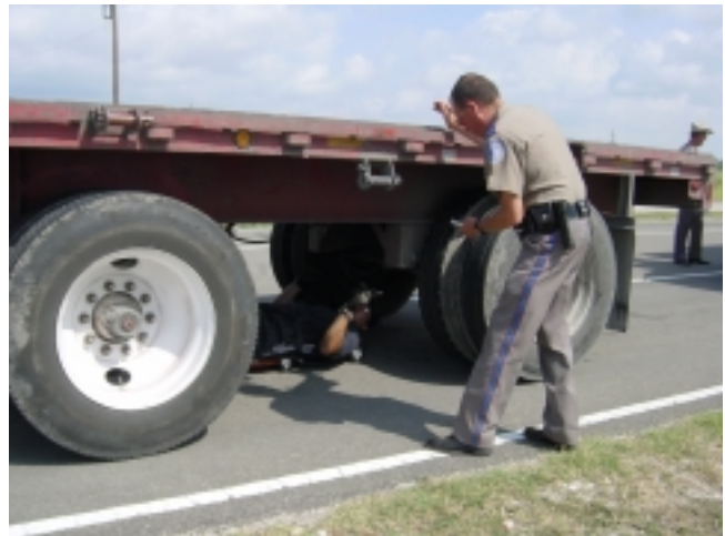
L&W troopers inspect brakes on a commercial motor vehicle during RoadCheck 2003.
